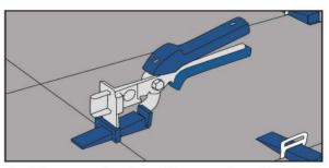
**4** - After squeezing the wedges together with adjustable pliers, the leveling process is complete. \*Do not squeeze more than needed.
