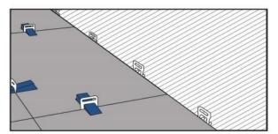
1 - After applying the tile to the thinset, the clip should be placed on the side of the tile. Also, their flat sides should be the same as the base.
