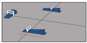
**3 -** Wedges must be manually inserted into the clip. Wedges must be manually squeezed and attached to the clip socket.
